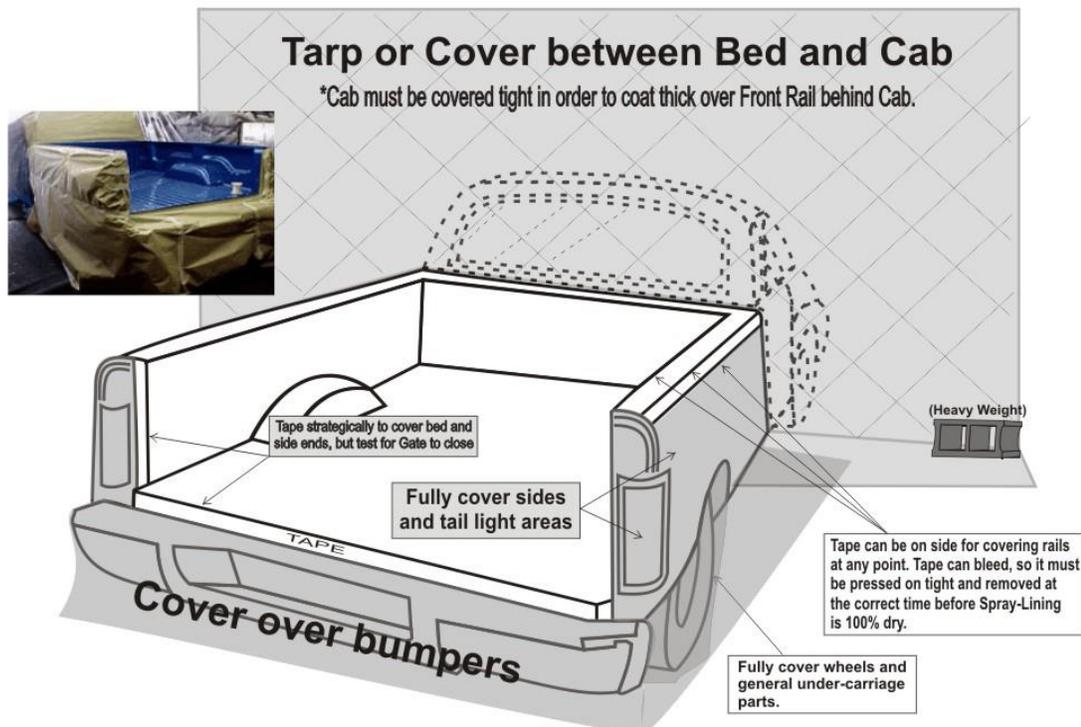
\* All tape & covers (tarps, paper or plastic) must adhere to each other & truck parts 100% with 0% openings or leaks.
